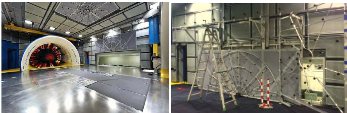
Figure 4. Pininfarina's wind tunnel: a) the 'top' and 'lateral' arrays [3], and, b) setup of the 'lateral', 'linear' & Univ.PM 'front' array.
