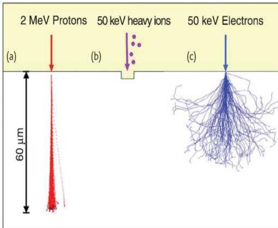
Comparison between p-beam writing, FIB, and (c) e-beam writing. The p-beam and e-beam images were simulated using SRIM and CASINO software packages, respectively.
