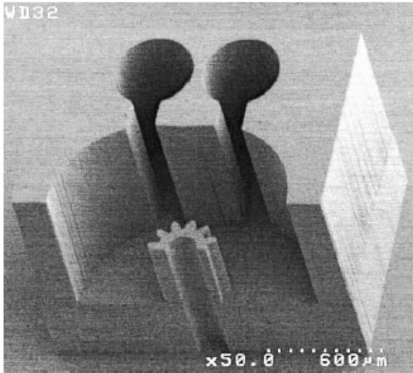
Three-level SU-8 structure with step heights of 300, 600 and 900 μm fabricated by X-ray lithography.
