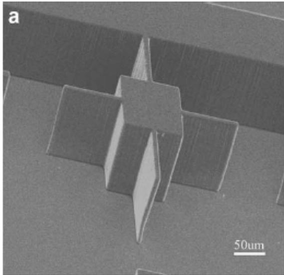
SEM photos of SU-8 microstructure with thickness of 400  $\mu\text{m}$ .
