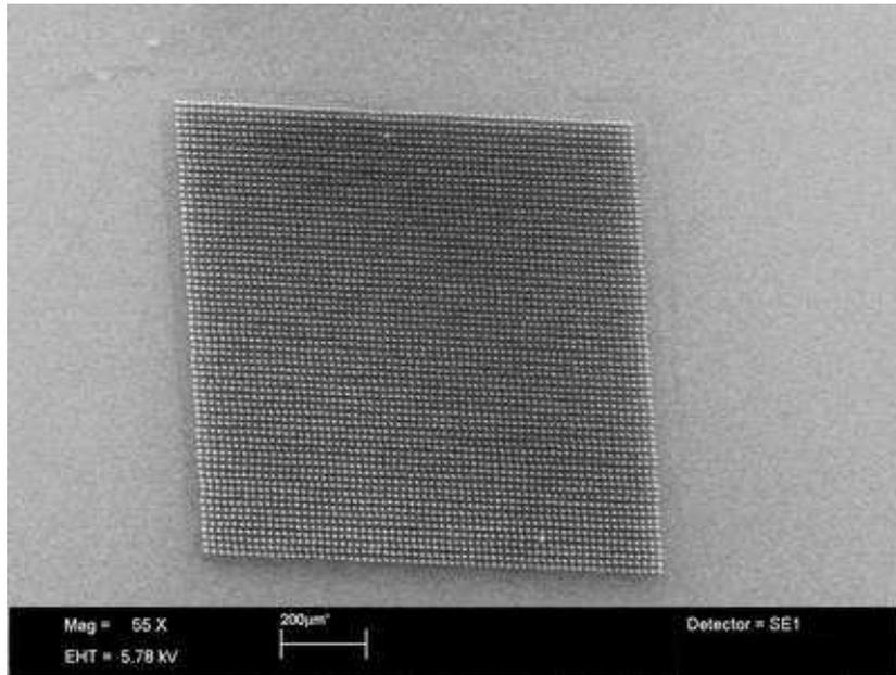
1 mm<sup>2</sup> area of single pixel irradiation on SU-8 (top view).
