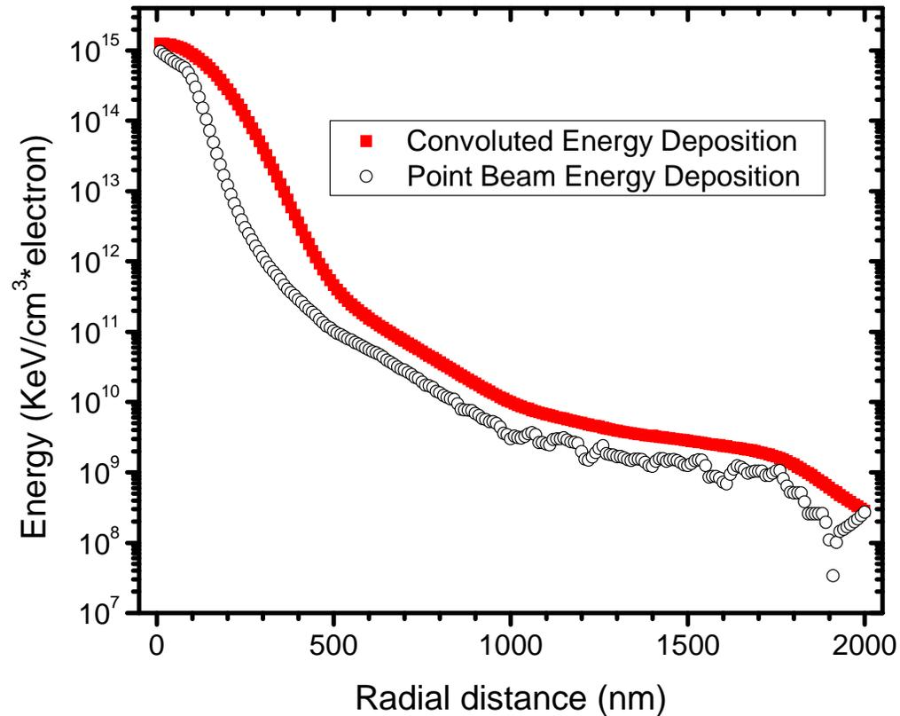
Energy deposition due to point beam and gaussian proton beam at the resist (10 $\mu$ m)/substrate interface (Beam diameter 100nm)
