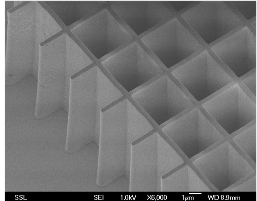
Side view of the pattern. Resist thickness  $12\mu\text{m}$ , aspect ratio: **42**. Beam size: 200nm in X-direction
