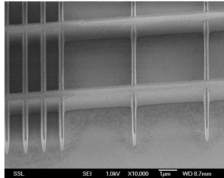
Top view of PBW double line irradiation on TADep resist.
