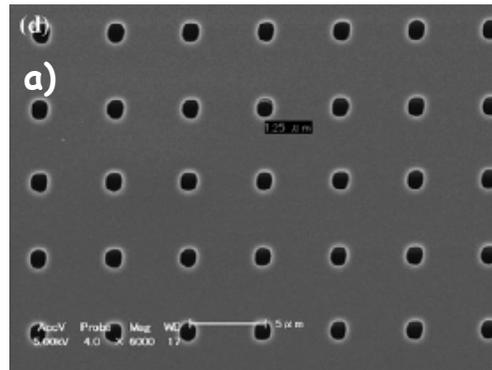
SEM image of 5-μm thick PMMA by PBW at 1.7 MeV (fluence: 100 nC/mm<sup>2</sup>) with writing patterns of dots (1.25μm diameter).
