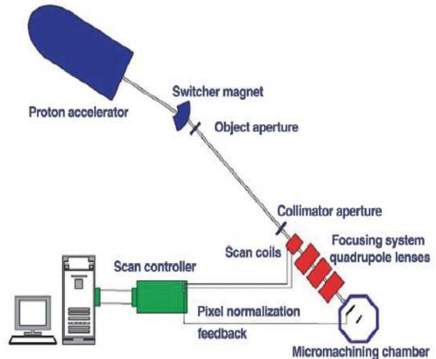
Schematic of the p-beam writing facility at CIBA. MeV protons are produced in a proton accelerator, and a demagnified image of the beam transmitted through an object aperture is focused onto the substrate material (resist) by means of a series of strong focusing magnetic quadrupole lenses. Beam scanning takes place using magnetic or electrostatic deflection before the focusing lenses.
