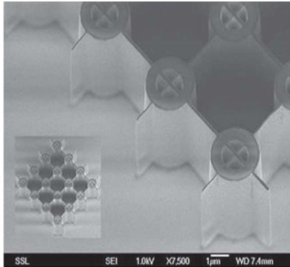
High aspect ratio test structures in SU-8 (60 nm wide, 10 μm deep structures).
