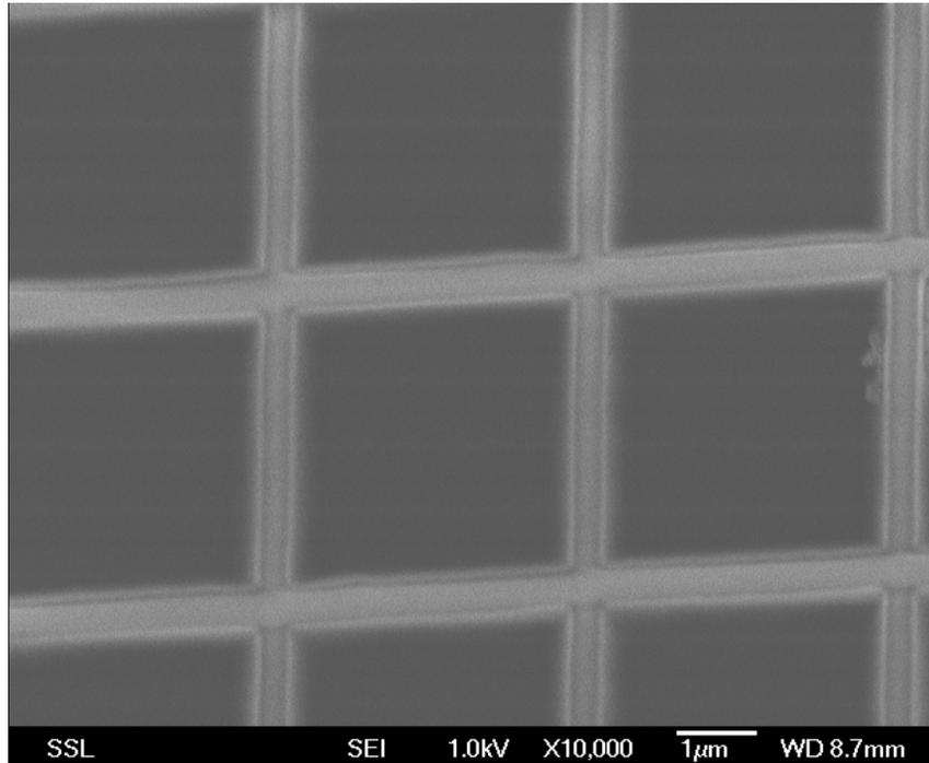
Top view of PBW double line irradiation on TADep resist. Line width **280nm** in X-direction.
