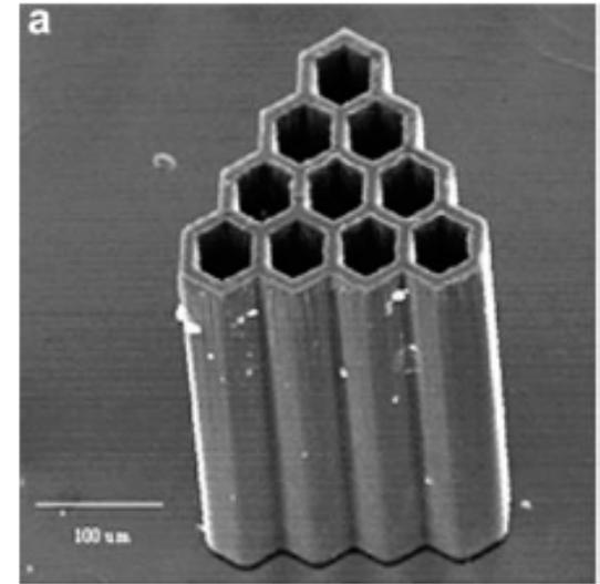
SU-8 patterns with thickness 210  $\mu\text{m}$ , width 10  $\mu\text{m}$
