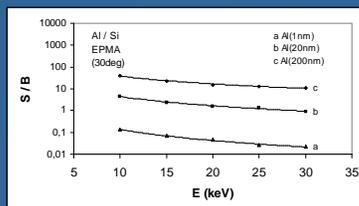
Figure 2b: Experimental values (EPMA) of the (S / B) ratio for Al/Si system and 30° angle of incidence.
