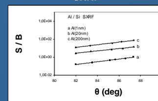
Figure 3: Experimental values of the S/B ratio in the case of back-foil XRF for Al/Si system and different film thicknesses as a function of the detection angle  $\theta$ .
