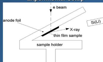
Figure 1a: Experimental setup used for back-foil XRF.
