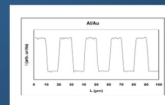
Figure 5: Line scan X-ray signal in the case of back-foil SXRF for Al/Au system. There is a pattern consists of 10um Al lines and 10um spaces on the backside of Au anode. The thickness of Al lines is 200nm.
