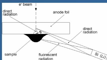
Figure 1b: Illustration of the trajectories of primary and fluorescence X-rays in back-foil XRF. The background is reduced by absorption of the continuous radiation, created by the electron beam, within the anode.
