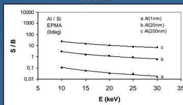
Figure 2a: Experimental values (EPMA) of the (S / B) ratio for Al/Si system and 0° angle of incidence.
