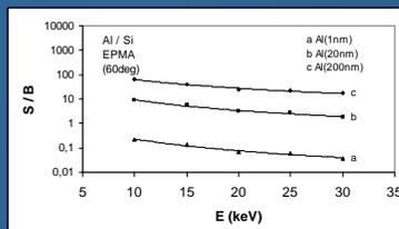
Figure 2c: Experimental values (EPMA) of the (S / B) ratio for Al/Si system and 60° angle of incidence.
