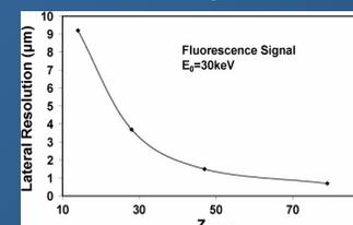
Figure 4: The lateral resolutions of the technique for various systems, as a function of the atomic number of the anode (Monte-Carlo calculations). The primary beam energy is 30 keV and the film thickness is 200 nm.
