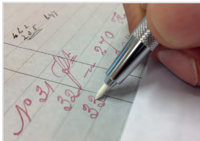
Fig 1: Sampling of a document from 1869. Red ink contains cochénille, the blue paper is dyed with indigo (© Birgit Reissland)
