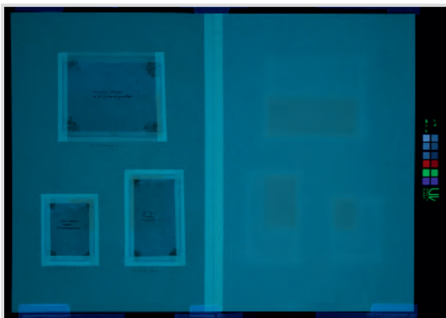
Fig 1: The Mondriaan Effect: an UV-photo of the brown discolouration in a print (Amsterdam City Archive Nr. K17) originating from the adjacent window mount (© Gauthier Patin & Frank Ligterink)
