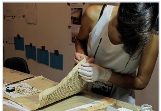
Fig 2: The enzyme dissolves the adhesive on the verso of the leaves, and the leaves can be separated easily (© J. Skou-Hansen and R. Buccarella, SMK)
