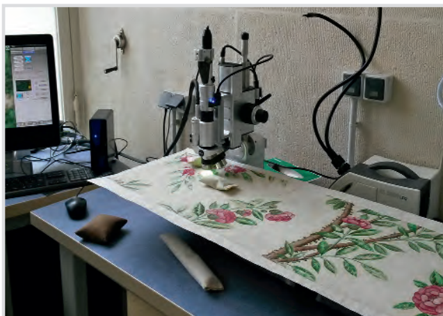
Fig 1: The 3D microscopy on Chinese wallpaper using the HIROX KH 8700 technology (© Julia Bischoff, 2015)
