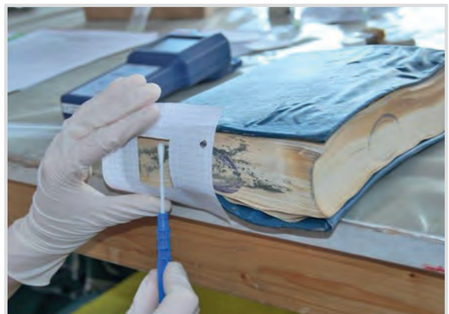
Fig 2: Measurement on a book edge to clarify the degree of contamination (© Meier-Wolff)
