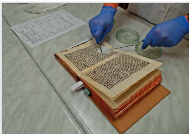
Fig 1: Impress sampling with Whatman filter paper (© Jakub Piechal)
