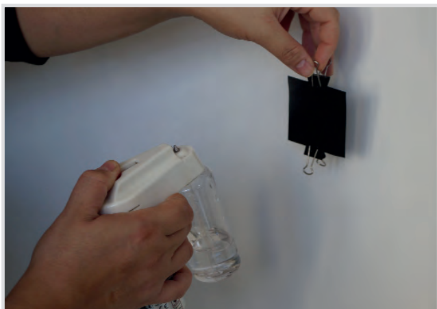
Fig 1: Application of a solution of gelatine on iron gall ink impregnated papers (© CRC)
