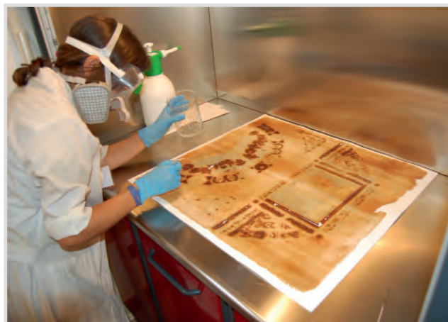
Fig 2: Spray- and brush application of the combined deacidifying-reducing solution on the back of the engraving (© AmbraD'Aleo)
