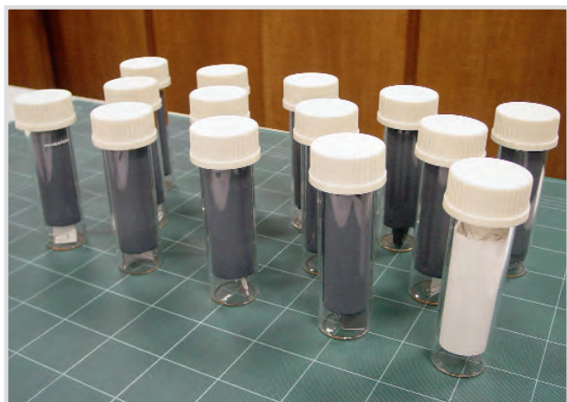
Fig 1: General view of the sample set before ageing. The blue paper is impregnated with an iron gall ink (© CRC)
