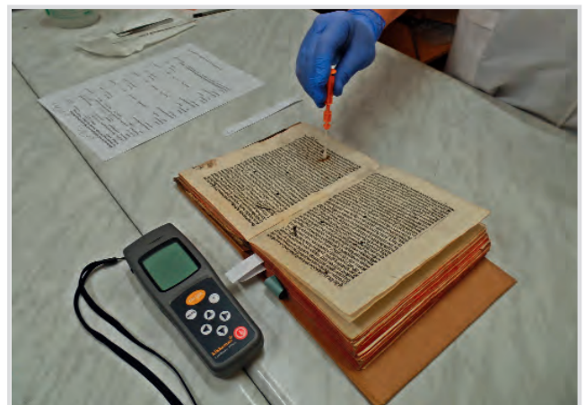
Fig 2: ATP sampling with kikkoman® Lumitester PD-20 (© Jakub Piechal)
