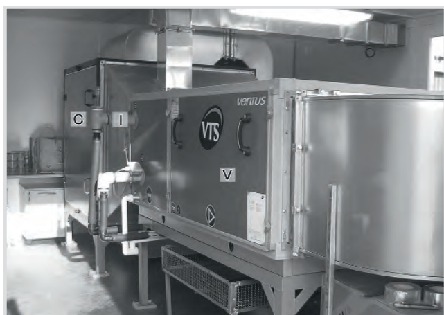
Fig 1: The chamber for silver nanoparticles misting, front (© Katarzyna Pietrzak)
