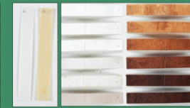
Fig. 4 Montval mock ups. Left: Non oiled and oiled mock ups before ageing. Right: From the top to the bottom, the mock ups at 1, 4, 7, 14, 21 and 28 days of ageing.
