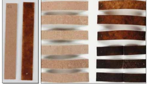
*Fig.* 4 **Kraft mock ups.** Left: Non oiled and oiled mock ups before ageing. Right: From the tope to the bottom, the mock ups at 1, 4, 7, 14, 21 and 28 days of ageing.
