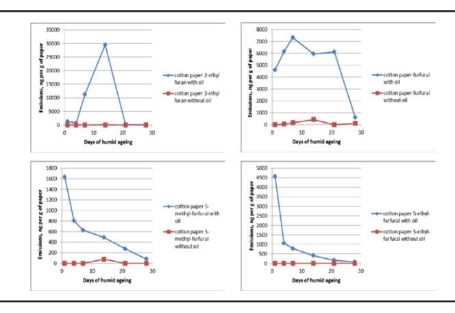
Figs. 21, 22 Graphs showing emissions of 2-ethyl furan, furfural, 5-methylfurfural and 5-ehtyl-furfural in ng per g of paper over 28 days, from cotton paper mock ups (left table) and wood based (Montval) paper mock ups (right table) with and without linseed oil application.
