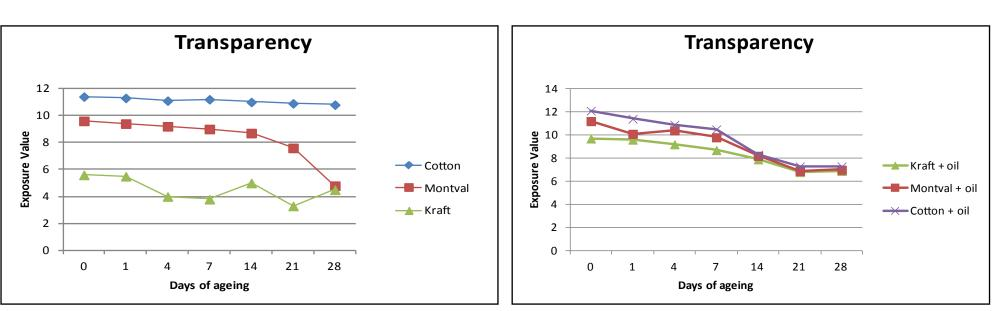
ageing. For the white colour papers the increase of the red colour, and the fluctuation pattern within that, could be indicative of the chemical changes. Also differences in colour through each mock up are strongly associated with the oil concentration on the paper locally.
