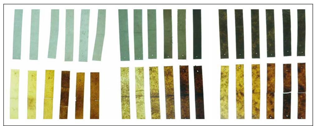
Fig. 6 Trasmitted light photography. Top row: sets of cotton, motval and kraft plain paper mock ups in 1, 4, 7, 14, 21and 28 days of ageing. Lower row: sets of oiled cotton, motval and kraft paper mock ups at all ageing periods.
