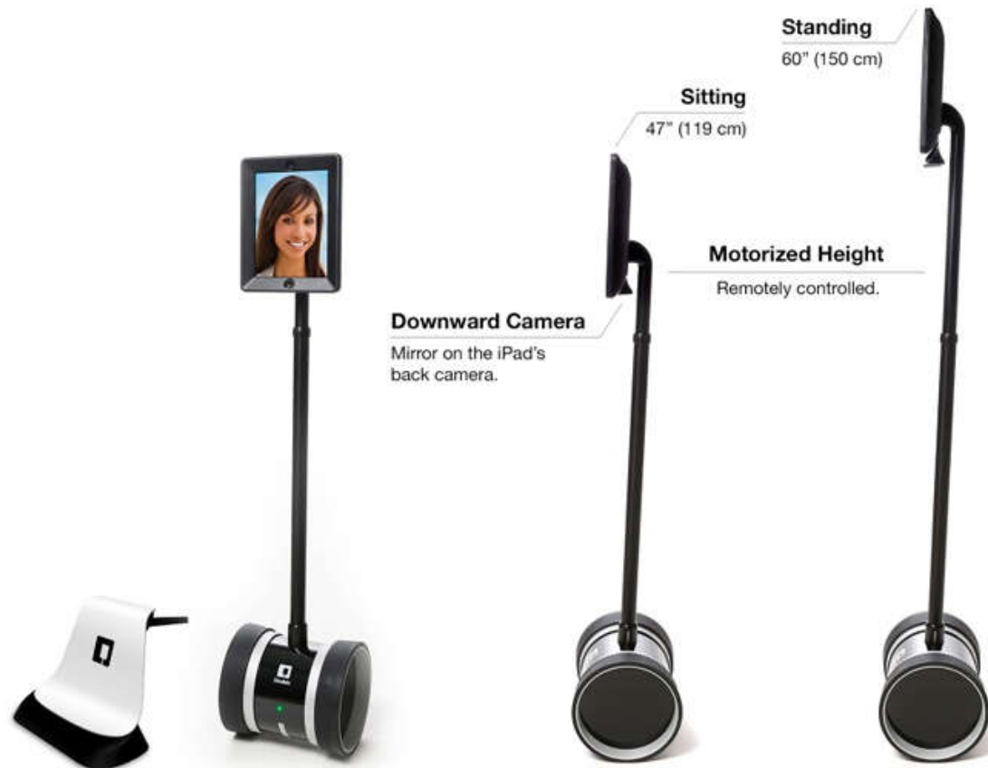
Figure 13.9: The Double telepresence robot is a screen and camera on a stick. The robot costs around $2500, and the screen is a tablet, such as an iPad. The height can even be adjusted remotely so that the person may appear to be sitting or standing.
