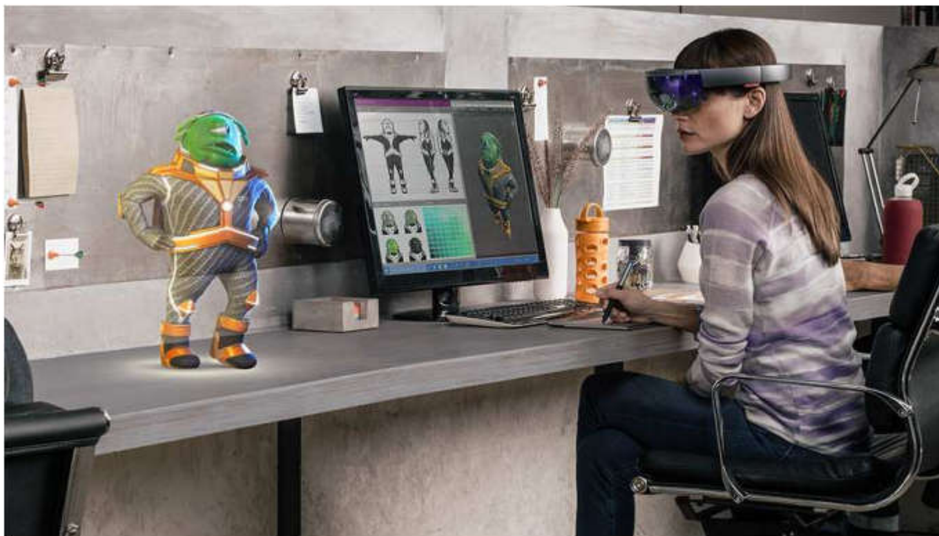
Figure 1.19: The Microsoft HoloLens uses advanced see-through display technology to superimpose graphical images onto the ordinary physical world, as perceived by looking through the glasses.
