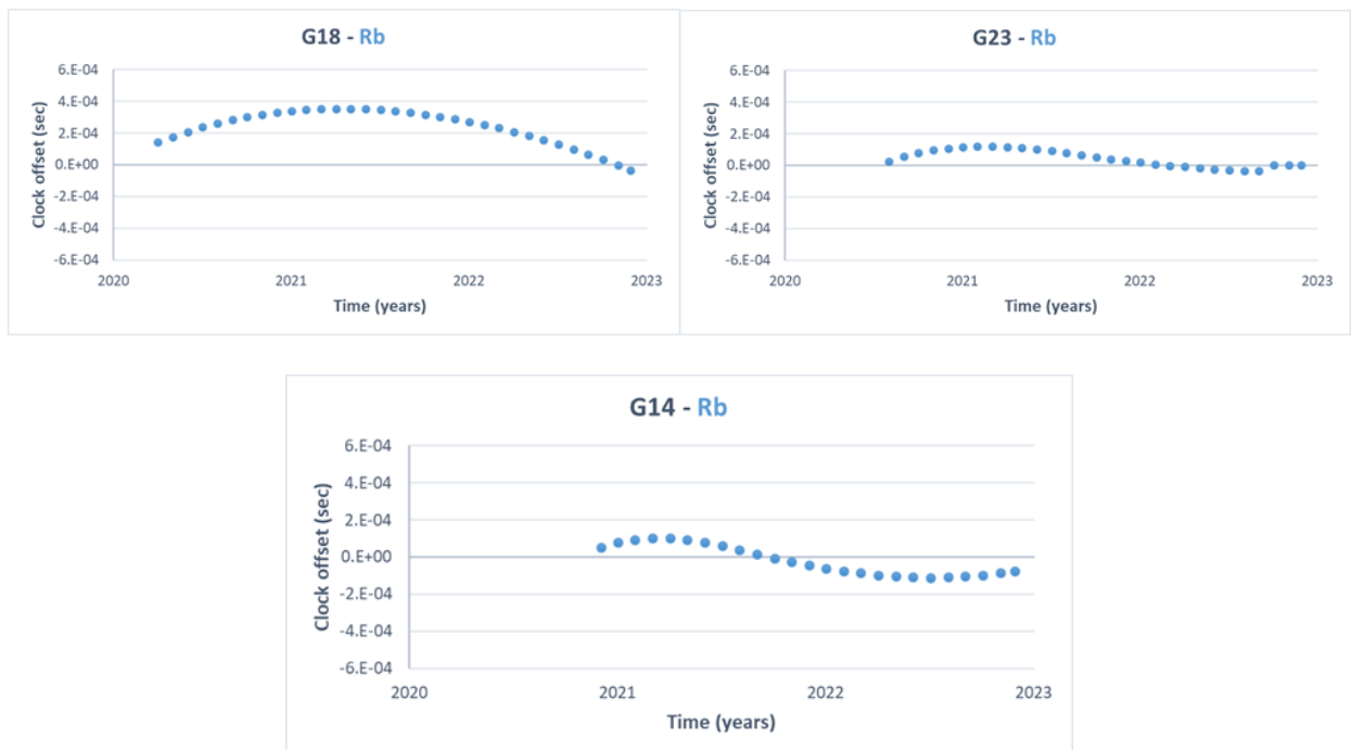
Fig. 6 Clock offset of GPS Block III satellites.
