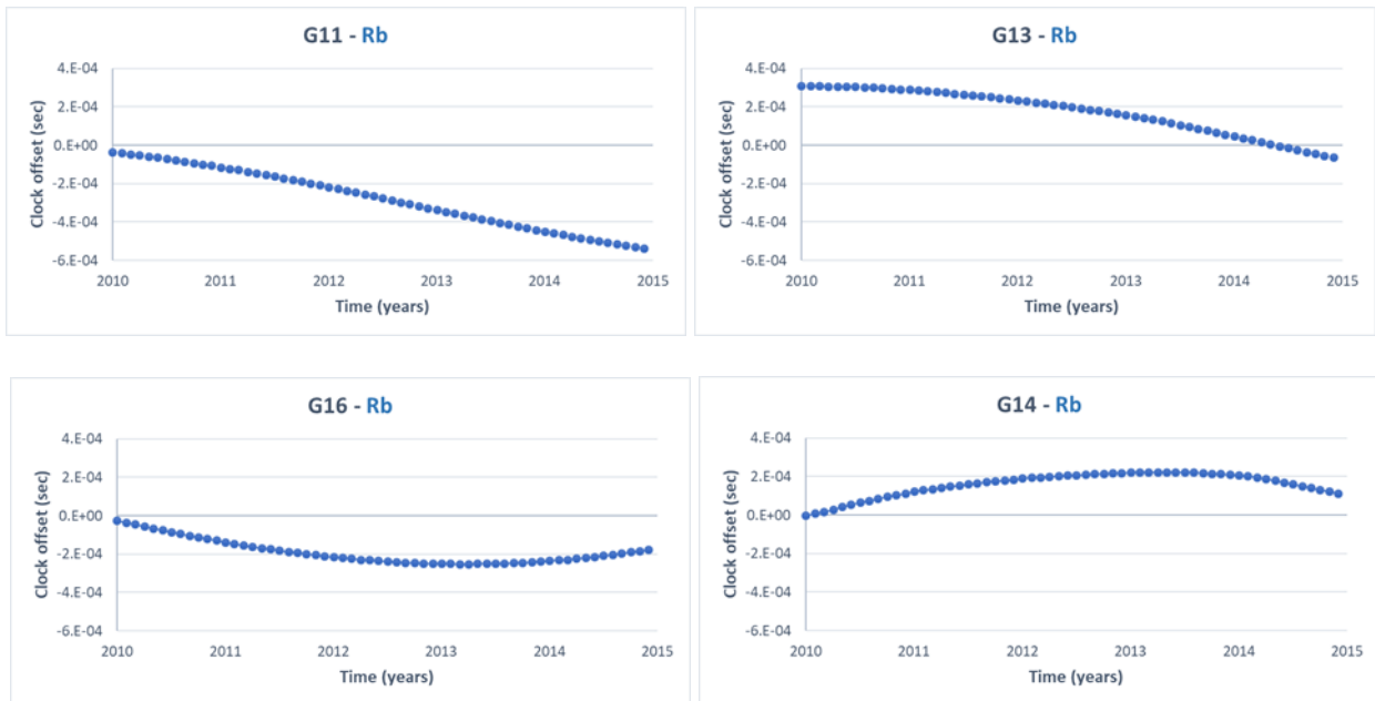
Fig. 2 Clock offset of GPS Block IIR-A satellites.
