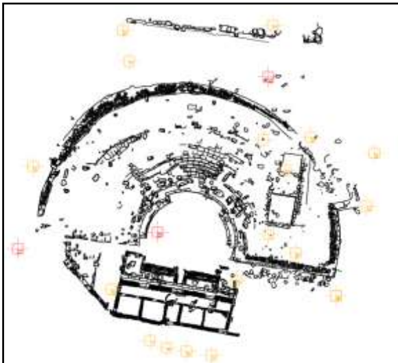
Fig. 1a. The ancient theatre of Thebes Fthiotidas with the positions of the geodetic network (red) and TLS (orange).
