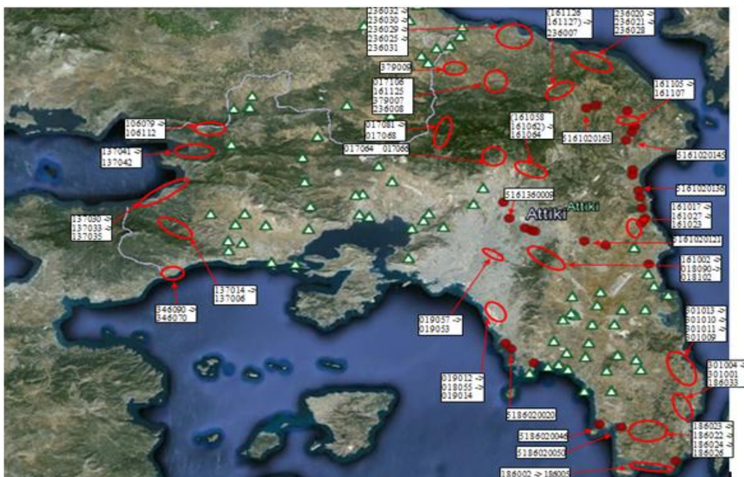
Figure 7: Map of the Attica test area, with the location of the groups of alternative benchmarks (red ellipsoids), the existing height benchmarks (red circles) and the already available benchmarks of the national trigonometric network (green triangles).
