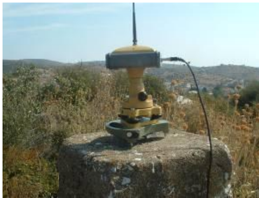
Figure 10: The TOPCON HiperPro receivers during the GPS measurements on BMs in Attica.
