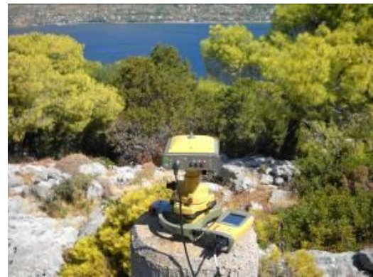
Figure 10: The TOPCON HiperPro receivers during the GPS measurements on BMs in Attica.
