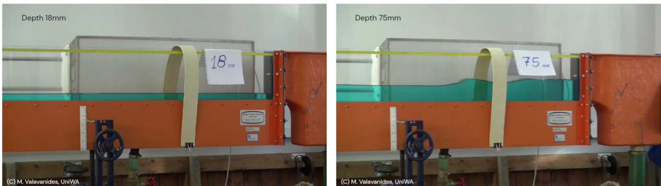
Figure 5: Experimental setups for measuring surface wave celerity at different water depths (left: 18 mm, right: 75 mm).
