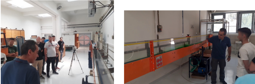
Figure 2: Laboratory reproduction of hydraulic phenomena along a six-meter flume at the new Hydraulics Lab, Campus 2. These sessions support theoretical instruction by illustrating fundamental concepts in open-channel flow.
