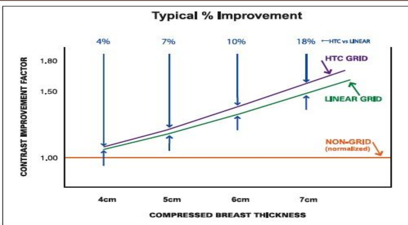
Figure 4. Contrast Improvement Factors for HTC and Linear grids are shown as a function of compressed breast thickness
